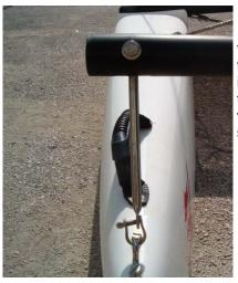
Identify the right side from the left side of the bar (look for the stickers) and position it the right way between the two hulls and attach the bar with the supplied shackles as shown on the photo.
