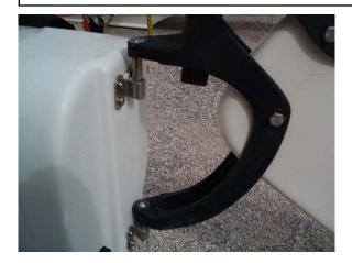
Identify the right rudder from the left rudder (look for the stickers on the rudder arms). As shown, line up the rudder pintles (metal pegs on the hulls) with the rudder castings. Push the rudder castings down onto the pintles.
