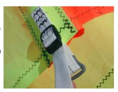
Using the straps and clips on the leech of the mainsail, secure each batten into it's respective pocket (as per photograph). Push the battens in reasonably hard - sufficient to remove any wrinkles from the pocket. NOTE: it is important to relieve the tension on the battens after each day's sailing. This will prolong the life of the sail.
