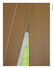
Unfold the jib and shackle the head onto the jib halyard with the shackle provided. Fasten the clip at the top of the jib to the forestay wire. Pull on the halyard and raise the sail, fastening each clip to the forestay in the process. When the sail is raised, shackle the tack of the jib to the adjuster on top of the
