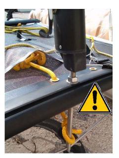
With the person on the trampoline supporting the mast, the other person takes the forestay and connects it to the stay adjuster fixed to the jib furler. Pin the forestay towards the top of the adjuster. Now, provided all the clevis pins have the split rings fitted, the mast is supported by the shrouds and
