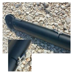
Remove the main and jib halyard lines from the ropes bags. Unroll the main halyard wire that is secured at the head of the mast. Using a bowline knot, secure the main halyard line to the thimble at the end of the halyard wire. Now, secure both ends at the base of the mast.
