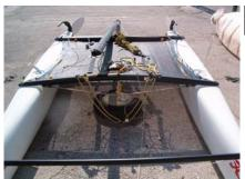
With the base of the mast facing towards the front of the boat, lay the mast on top of the boat. (place some pading under the mast to prevent scratching).
