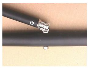
Locate the tiller extension and secure it to the tiller crossbar using the clevis pin and ring clip provided.
