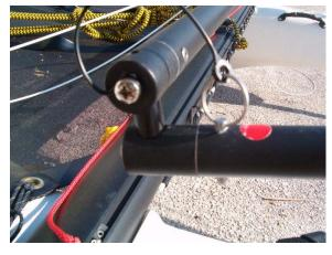
Locate the tiller crossbar and identify the left and right hand ends. NB: the tiller crossbar (1) locates on top of the tiller/rudder arms (2).
