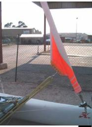
The jib can now be furled by pulling on the furler line and cleating it off in the jam cleat. The jib will not furl fully if the jib sheet is cleated on.
