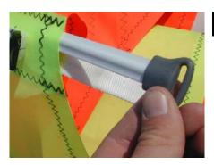
Unfold the mainsail and lay on a flat clean surface. Undo the set of battens and identify which batten goes in which batten pocket. Insert the battens into the pockets.
