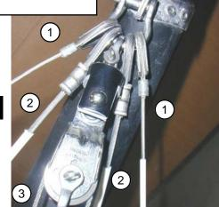
Remove all the wires from the wires bag and unroll them. They are all already mounted on the 8 mm shackle. Ensure that all twists are removed.
