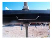
Unfold the trampoline. Note that the side tension lines are prethreaded. Insert the front sealed bolt rope edge into the trampoline track of the front crossbar. Continue feeding the trampoline into the trampoline track and position it in the centre. Line up the grommet in the centre of the front edge of the trampoline with the dolphin striker post. This will position the
