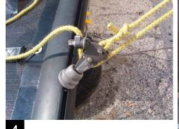
Attach the jib clew blocks to the clew of the jib using the snap hook provided.
