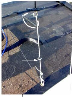
The height of trapezing can be adjusted by changing the position of the rope lock.
