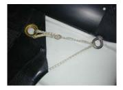
Tensioning the sides: starting at the right rear corner, take the line that emerges from the trampoline. Lead it through the eye strap on the rear beam and then through the grommet/eyelet. Tie it off with a bowline knot or similar.
