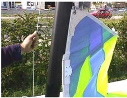
Now, pull on the main halyard line whilst feeding the sail into the track cut out.
