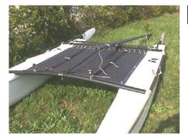
With the base of the mast facing towards the front of the boat, lay the mast on top of the boat. (place some pading under the mast to
