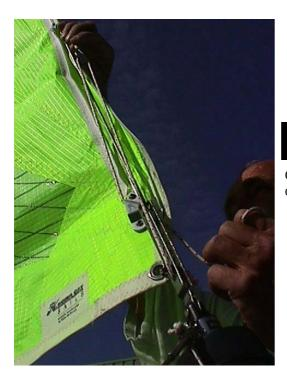
Shackle the jib head to the jib halyard. Then positi the jib and the halyard line against the forestay. Close the zipper ensuring that the halyard line remains inside the zipper. As you pull down on the halyard line close the zipper as the sail is raised.
