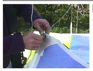
Place the sail on the trampoline, the battens clips towards the back. Undo the main halyard wire from the mast and shackle it to the head board of the mainsail. Now, feed the bolt rope at the head of the sail into the cut out in the sail track on the mast.
