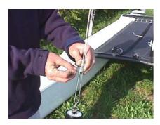
10 With the person on the trampoline supporting the mast, the other person takes the forestay and connects it to the stay adjuster fixed to the jib furler. Pin the forestay towards the top of the adjuster. Now, provided all the clevis pins have the split rings fitted, the mast is supported by the shrouds and forestay.
