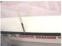
Next, fasten the shrouds into the stay adjusters. To begin with, fasten the shroud about half way up the adjuster. This position can be adjusted later. The position influences mast rake. Now fasten the twist toggles to the anchor bar pins on each side of the boat. You can pull the cover partially over the stay adjusters at this time. The assembly of the trapeze wires can wait until after you have raised the mast.
