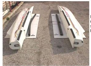
Position the hulls parallel on the ground approximately 1,5 meter apart. Have the front and rear crossbar ready. With the supplied spanner, unscrew the parts that are fixed onto the hulls.
