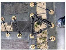
Temporarily tie off the line at the aft end, then remove slack again by working it out front to back. Lace the two aft lines simultaneously in the same manner.
