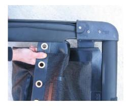
Insert trampoline half into the flared sidebar track so that the grommets are running down the center and across the back. Position the forward edge even with the forward crossbar. Insert the forward edge of the trampoline into the front cross bar track adjacent to the corner casting and slide it all the way to the center. Repeat this operation for the opposite side. Install the aft lacing strip by feeding the larger bead into the track in the aft crossbar. Make sure it is centered.
