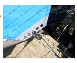
of the opposite jib block on the front crossbar, then between the sheaves, then through the 2nd hole of the Trentec traveller car (the one towards the inside) from outside to inside, and then back to the first hole of the traveller from inside to outside. Secure the end of the line with a knot.
