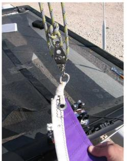
Take the jib block at the bottom of the mast and fix it to the head of the jib. The small line on the jib is a further security.
