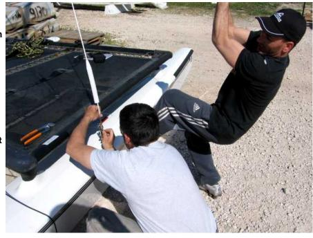
one of the shroud to the four or fifth hole of the stay adjuster. Have someone pulling down on the trapeze in order to relieve the shroud. Do the same operation on the opposite side. Caution: it is necessary to have the same tension on both sides. Then put the shrouds covers completely over the stay adjusters.
