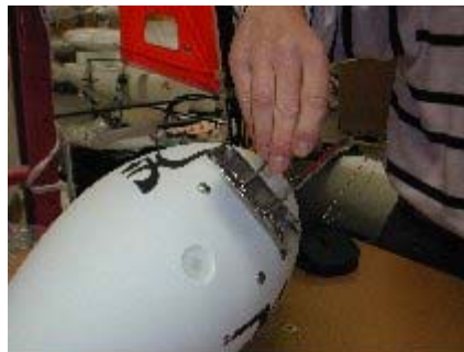
2- Adjust the alu plate so that the holes fit the four holes on the device and fix it with the screws.
