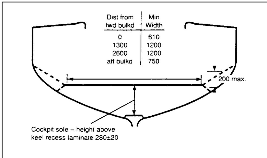
bonding the cockpit sole to the hull. Such flange (if any) shall not extend more than 50mm above the cockpit sole at its highest point nor itself measure more than 100mm at any point. The cockpit sole moulding may incorporate the forward and aft bulkheads and in this case flanges not exceeding 50mm wide bonding the bulkheads to the inner surface of the hull are permitted.
