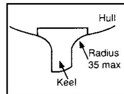
E.3.3.2 The athwartships radius in way of the keel-hull joint shall not exceed 35mm.
