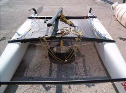
**6** With the base of the mast facing towards the front of the boat, lay the mast on top of the boat. (place some padding under the mast to prevent scratching).
