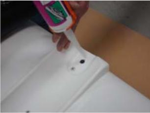
**2** Lift the right hull into an upright position. One person straddles the hull to hold in position. The other one applies the silicone sealant (for waterproofing) around the bolt holes and on rivets.
