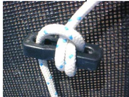
The height of trapezing can be adjusted by changing the position of the rope lock.
