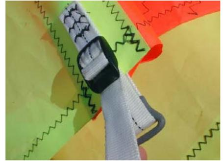
**2** Using the straps and clips on the leech of the mainsail, secure each batten into it's respective pocket (as per photograph). Push the battens in reasonably hard - sufficient to remove any wrinkles from the pocket.
