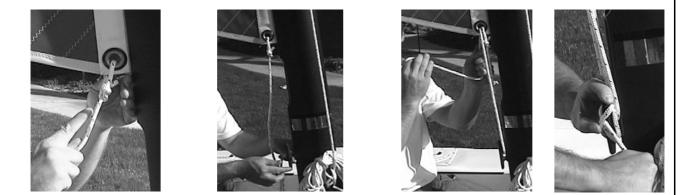
Tie the downhaul line to the grommet at the bottom of the main sail nearest the mast. Use a bowline knot. Pass the line down and through the downhaul cleat located in the mast track. Pass the line back up and through the downhaul (tack) grommet. Using the 3:1 purchase this creates, tension the luff of the sail until the sail looks smooth and horizontal wrinkles are removed. Tie off the line at the cleat.
