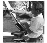
2 The jib is furled on the forestay and covered by a snorkel. To remove the snorkel, simply unzip as it is pulled down.
