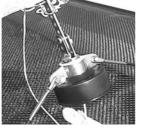
2 Insert the forestay adjuster into the furler drum one or two holes and pin in place. Fasten the jib luff wire to the forestay adjuster.
