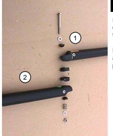
Locate the tiller crossbar and identify the left and right hand ends. NB: the tiller crossbar (1) locates on top of the tiller/rudder arms (2).
