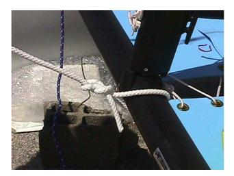
Take the righting line from the rope bag and attach it to the front crossbar as indicated on the picture. Store the excess line in the trampoline pocket.
