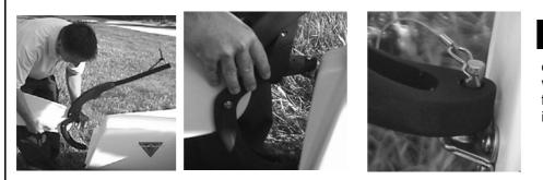
2 Insert the retainer pins to lock the rudders in place. The pins will prevent the rudders from falling off the boat in the event of a capsize.
