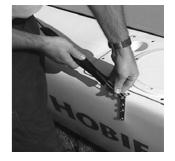
4 Attach the furler to the two bridle wires. Make sure the hole in the furler housing points towards the front crossbar. Wind some line onto the furler drum - 10 turns or so.
