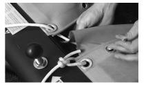
2 Tie a bowline knot to the forward left/port grommet in the trampoline. Pass the line through the opposite grommet, top/down and then through the lacing flap. Come up through the next (left) grommet and then continue to lace towards the aft of the trampoline following this pattern (down through the right grommets and up through the left grommets). Keep the laces loose at this time. Lace as far aft as the line will go.
