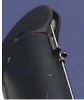
As shown, shackle the halyard to the top of the sail. Feed the top portion of sail into the mast track opening. Begin pulling on the halyard line. Use caution to be sure the sail feeds smoothly into the mast while raising. When the sail is all the way up, position the stopper on the wire halyard so that it engages in the halyard lock. Attach the main halyard rope to one of the white cleat at the bottom of the mast.
