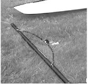
3 Insert the crossbars into one hull. See that the crossbars seat fully into their sockets in the hull.
