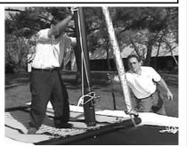
Ensure that the wires fixed on the mast are well positionned and not twisted. Stand on the trampoline near the rear crossbar and lift the mast to your shoulder. Walk forward while lifting the mast until the side shrouds go tight preventing the mast from further forward movement. Lean your weight against the mast to hold it in this position.
