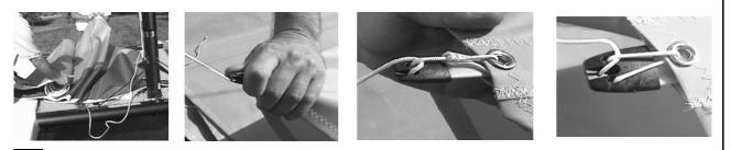
1 Unfold the sail on the trampoline. Insert the battens into the batten pockets. Fasten each batten as shown on the photos above. To tension the battens, pull tension on the line forcing the batten into the pocket and cleat it. Tension each batten so that the wrinkles in the batten pockets are removed, but not excessively otherwise the sail may be more difficult to handle. Release the tension at the end of the day to avoid stretching the sail while it is not in use.
