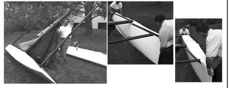
5 Be sure the forward spreader is fully seated in both hulls.
