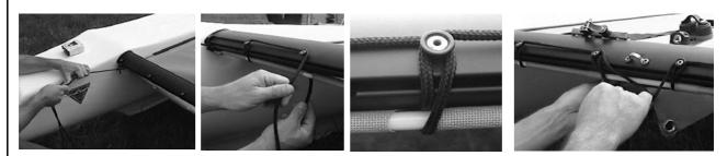
Pull the lace lines under the cross bar and tight. Begin the aft lacing by routing the left line up and over the first lace peg. Cross over to the next peg then down and around the rod. Pull the lace line tight then up and over the peg and then over to the next one and so on... Then start with the right and work towards the
