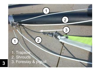
Remove all the wires from the wires bag and unroll them. Ensure that all twists are removed. Locate the 8 mm tang shackle and shackle the 5 wires to the mast tang, as per photograph above. Ensure that the shackle is tightened securely.
