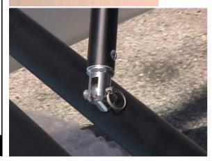
**3** Locate the tiller extension and secure it to the tiller crossbar using the clevis pin and ring clip provided.
