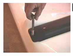
Insert the two bolts through the holes in the deck. Position anchor bars under gunwhale lip so that threading will commence and tighten both loosely using #14 wrench.
