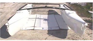
After both beams are in place, tighten all eight bolts securely.
