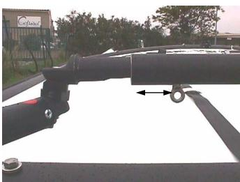
Assemble the stay adjusters with twist toggles, clevis pins and split rings. Attach them to the anchor bar pins. Ensure that the stay adjuster points fore and aft - as per photograph.
