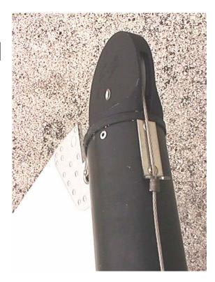
When the sail is all the way to the top of the mast, engage the slug on the halyard wire into the halyard lock. Secure the halyard line to the cleat on the side of the mast. Stow the excess line in one of the trampoline pockets.
