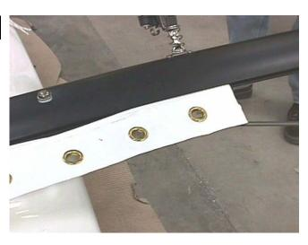
Identify the right and left side trampoline halves and insert them into the trampoline track in the back of the rear crossbar. Pull them all the way to the deck edge.
