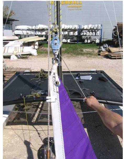
Secure the plastic hank to the forestay by twisting it 90° onto the wire and hoist the jib. Secure the jib halyard on the cleat at the bottom of the mast and stow the excess line on the trampoline pocket.
