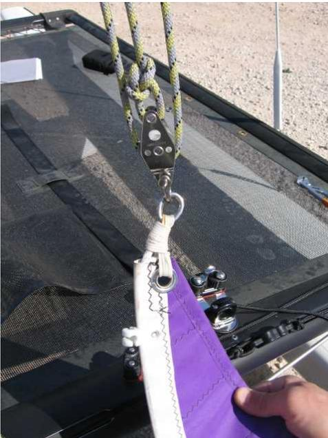
**5** Take the jib block at the bottom of the mast and fix it to the head of the jib. The small line on the jib is a further security.
