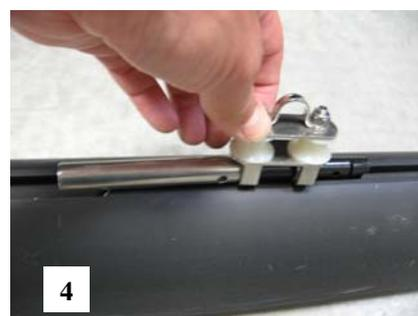
Reassemble the traveller car in a reverse manner, i.e. : fit in the upper part, slide the cylinder and place the pin and the split ring.
