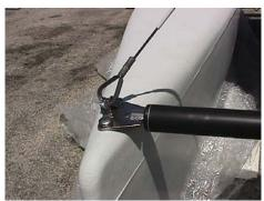
Before installing the jib on the Hobie Wave, you must first install the parallel bow spreader (provided with the turbo kit). Install bow spreader tangs on each bow under existing bridle wire tang as shown. Pin faces towards center. With trampoline loosened, place bow spreader in position on pins installed on bows.
