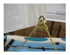
Before stepping the mast, Install jib halyard block on pig tail and place pigtail on the shroud shackle next to forestay wire. Run the halyard through the halyard block and tie off ends at lower cleat. Install halyard shackle. Step the mast.
