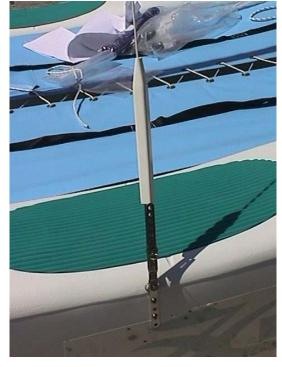
Next, fasten the shrouds into the stay adjusters. To begin with, fasten the shroud about half way up the adjuster. This position can be adjusted later. The position influences mast rake. Now fasten the twist toggles to the anchor bar pins on each side of the boat. You can pull the cover partially over the stay adjusters at this time. The assembly of the trapeze wires can wait until after you have raised the mast.
