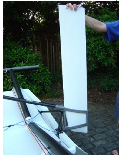
66. Insert the rudder blade to the stock. Friction will keep it up.
