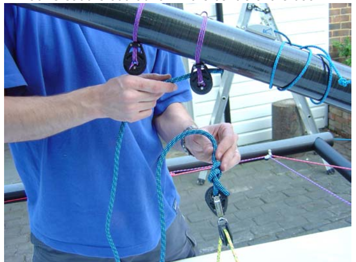
32. Rig the mainsheet starting with a bowline on the block attached to the mainsheet bridal. Then thread it through the front block on the boom.
