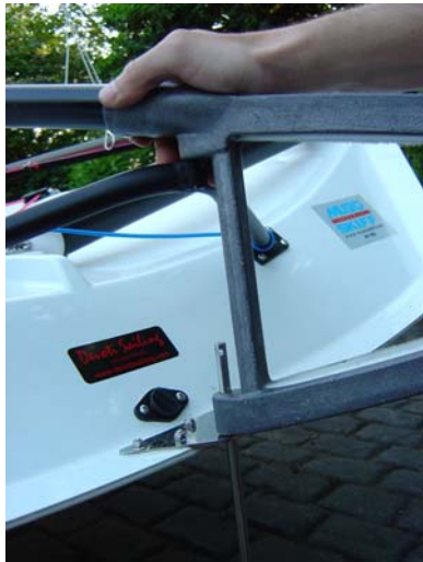
63. Offer the stock up to the pintles and insert the pintle bar from the bottom
