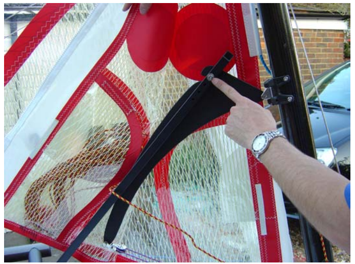
80. The bolt is usually in the top of the four available holes.
