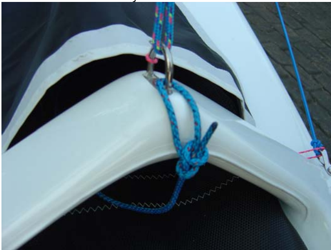
49. Tie the halyard onto the forestay eye, otherwise the elastic will pull it back again.
