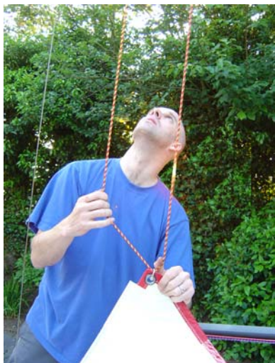
69. Check the halyard doesn't have any twists and shackle the head on.
