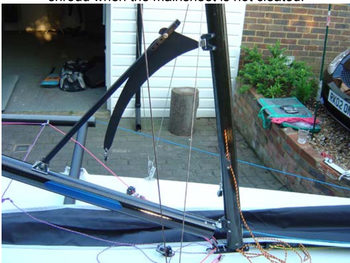
37. Locate the two kicker bars together. Note if they will not then just adjust the height of the boom by adjusting the angle of the boom with the main halyard.
