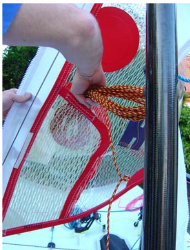
72. Coil the halyard up and post it in the pocket on the starboard side of the main.
