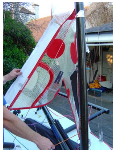
71. Once it is at the very top give the halyard a good pull and cleat it off.
