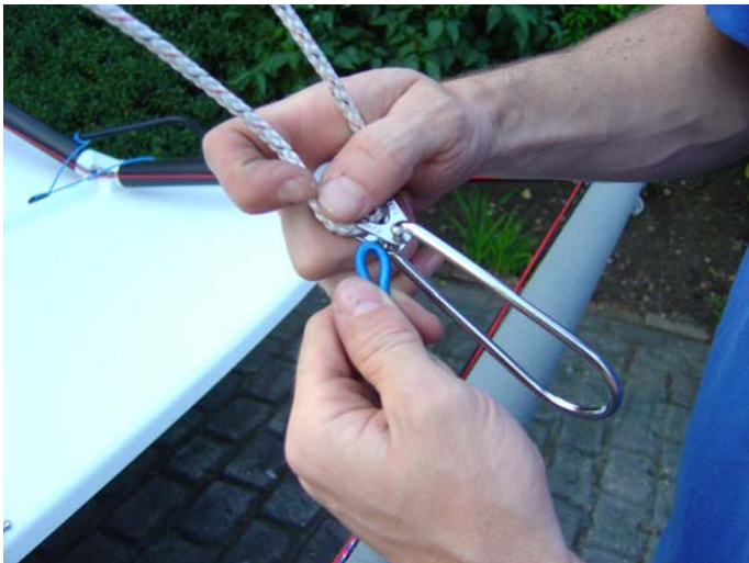
23. Now the rig is tensioned the trapezes can be connected to the elastic that is available on the wing bar.
