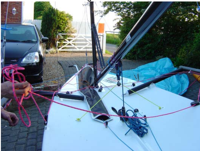
55. Make sure you have run the kite sheets on top of all other ropes and behind the mainsheet.
