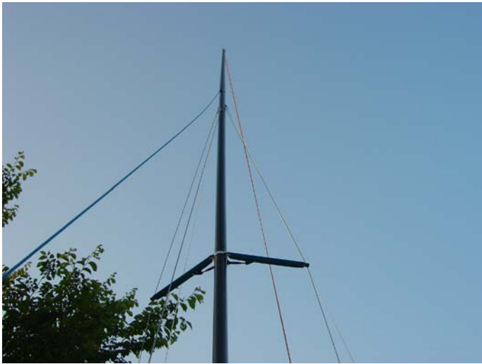
61. Have a quick look up to make sure the halyard is not twisted.
