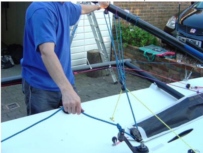
35. Pull the sheet on a little bit and put a stopper knot of your choice into the mainsheet. This will stop the boom hitting the shroud when the mainsheet is not cleated.
