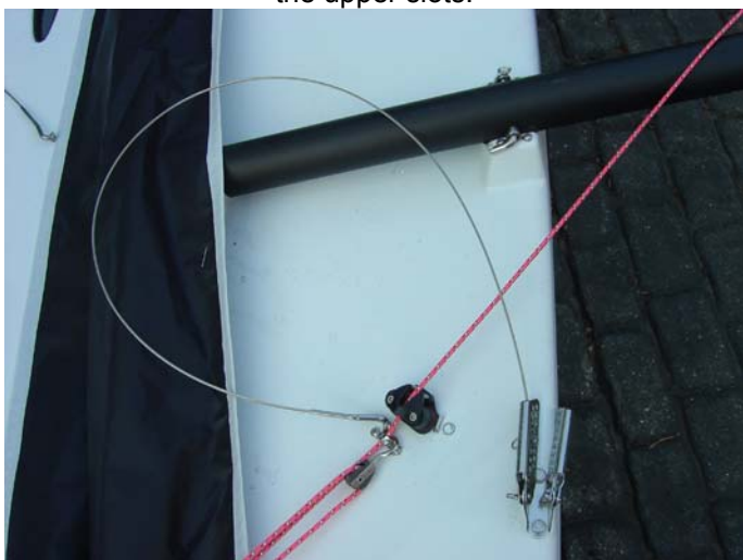
17. Attach the lower shroud to the inboard rig adjuster. Five holes down on the front row is a good start but check www.mustoskiff.com for tuning information
