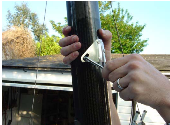
20. With the weight of the mast now on the trapezes attach the lower shrouds to the plate on the mast. Do both sides and the mast will now be self supported.
