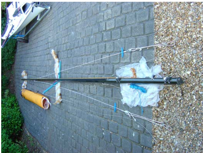
15. Before stepping the mast lay it out (on padding, you don't want to scratch your new carbon mast) and check that all the line and wires are not twisted up. Also look up and check you are not going to hit anything with the mast when you raise it, especially power lines!! NOTE: The trapeze T terminals go in the upper slots.
