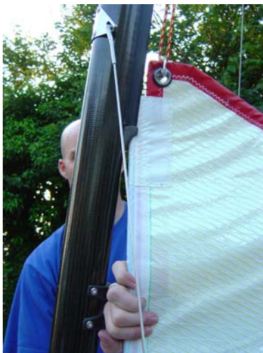
70. Slowly pull the main up, as it's fully battened it can be stiff so go steady. A good spraying on McLube on the track can make things easier.
