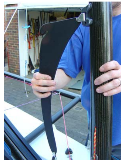
36. Fit the other kicker bar to the upper gooseneck.
