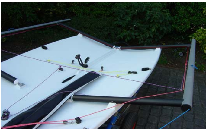
14. With the wings fitted ensure that the line for the downhaul (pink in this picture) is on top of the wing bar.
