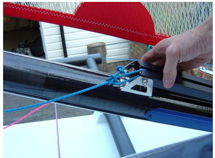
78. Tie the slack end of the outhaul to the bolt of the kicker bar to keep the end tidy.
