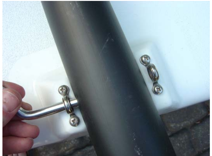
11. Insert the wing pins. If they are difficult to insert you may not have the wings in properly. Give them a little "wobble" until the pin can be inserted.
