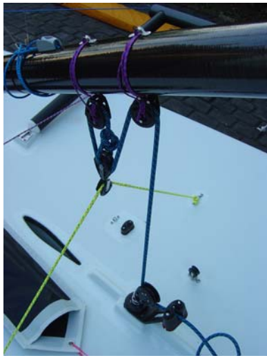
33. Then thread it through the block on the boom then back through the aft block on the boom and through the jammer. MAKE SURE YOU GET IT THE RIGHT WAY THROUGH THE RATCHET BLOCK,
