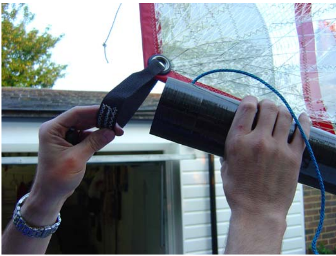
74. Post the clew strap over the end of the boom.
